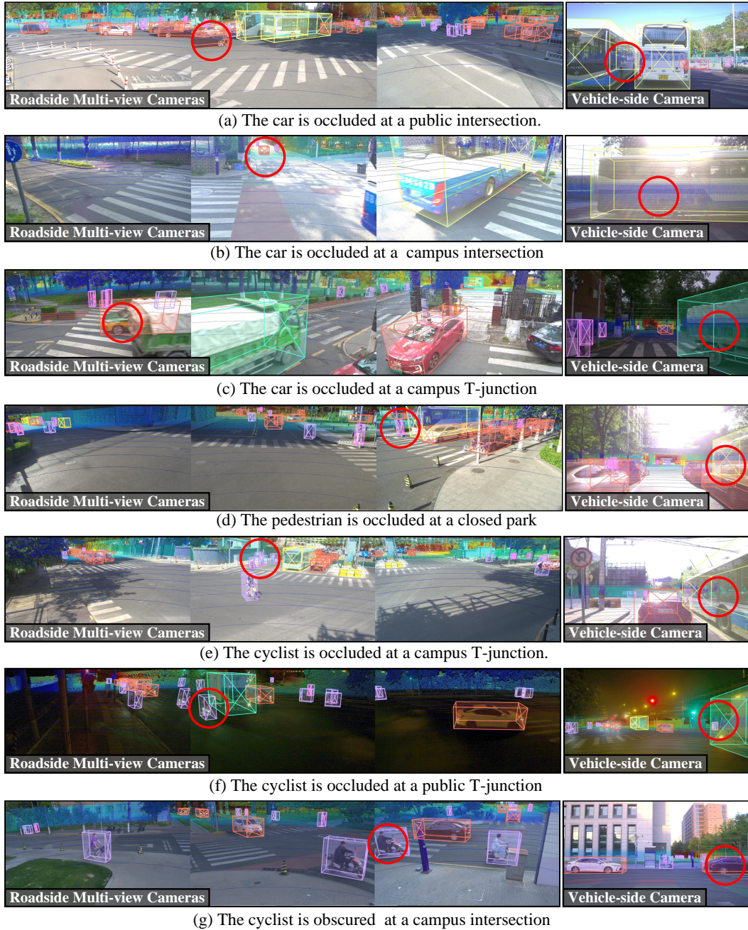
Figure 10: Diverse corner cases for single-vehicle autonomous driving. Each case is depicted by roadside multi-view images on the left and the vehicle-side image on the right. We use a red circle to mark the occluded objects. The red circle highlights critical objects that are occluded from the vehicle-mounted perspective but remain observable from the roadside viewpoint.
