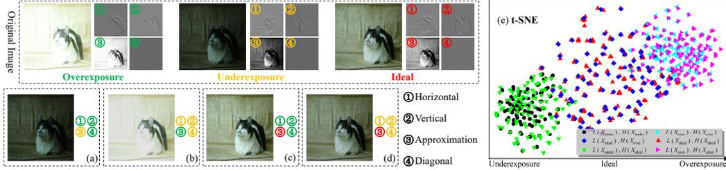
Figure 3: After Haar DWT decomposes an image, swapping its low-frequency component (③) with the high-frequency components (①②④) of the same image under different exposures produces visually similar results (a-d) as well as similar t-SNE features (e).
