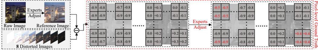
Figure 7: Overview of the proposed IEA dataset annotation process. First, collect images of different exposure conditions and then adjust the raw image by experts to obtain reference image; Second, calculate exposure residual between the reference and 8 distorted images, and then have experts adjust the local exposure residual. The closer it is to -1, the more overexposed the corresponding pixel is; and the closer it is to 1, the more underexposed the corresponding pixel is.
