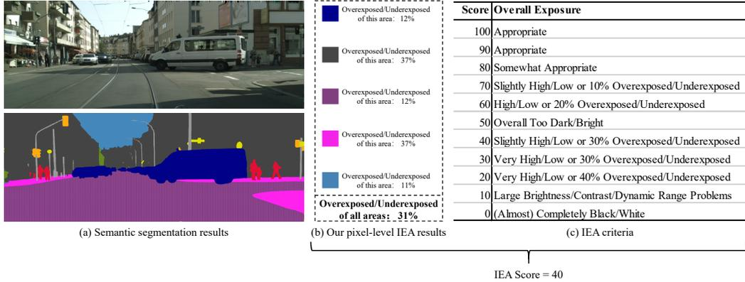
Figure 9: Based on the IEA criteria provided by different manufacturers, our pixel-level IEA results can be mapped to the corresponding IEA scores according to the provided criteria without fine-tuning.
