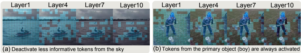
Figure 6: Visualization of activated tokens. We present two representative samples from the K400 dataset. Blue patches represent the tokens activated in token dispatcher (Detailed in Section 3.2). Results verify that the token dispatcher has learned to identify informative tokens during fine-tuning.
