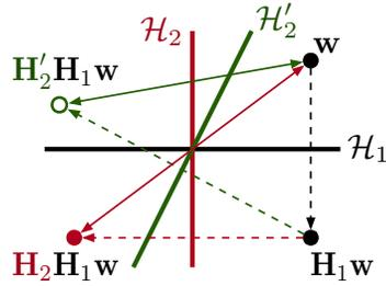
Figure 2: A 2D illustration indicating that when the reflection planes  $\mathcal{H}_1$  and  $\mathcal{H}_2$  are orthogonal, the distance  $\|\mathbf{H}_2\mathbf{H}_1\mathbf{w} - \mathbf{w}\|_2$  is maximized.
