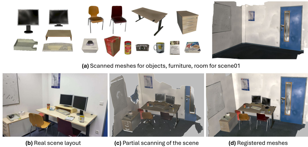
Figure 4: Example for the Scan and Register Step. (a) We pre-scan all meshes in the scene before setting up the scene. This ensures that all objects and furniture are scanned in a high quality, water-tight manner. (b) Then we place the furniture in the room to setup the scene and (c) scan the entire scene (Note that the scene is not scanned completely), such that we can (d) register all pre-scanned meshes to the scene layout via manual correspondence selection followed by ICP.
