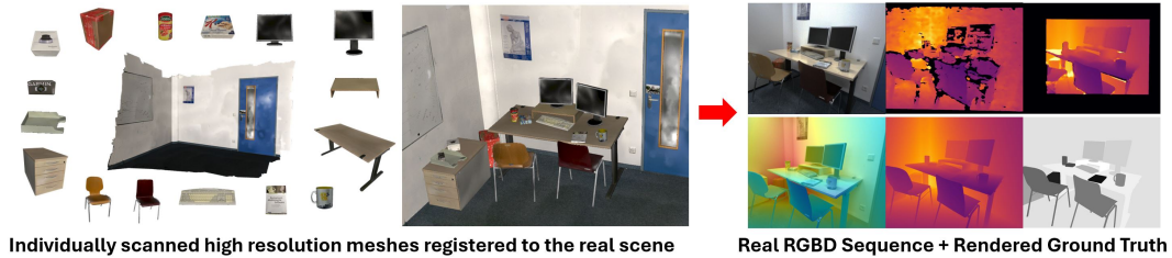
Figure 1: Due to the typical acquisition pipelines, traditional indoor 3D datasets can provide incomplete meshes for their scenes with missing structures and holes. Our dataset annotation pipeline, in contrast, starts from scanning individual objects in a high resolution manner and then registers them to the real scene and real camera sequence allowing highly detailed ground truth rendering for dense 3D vision tasks.
