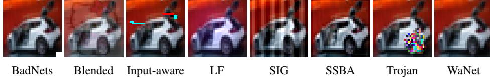
Figure 7: Examples of 8 backdoor-attack triggers on the same image of CIFAR-10.
