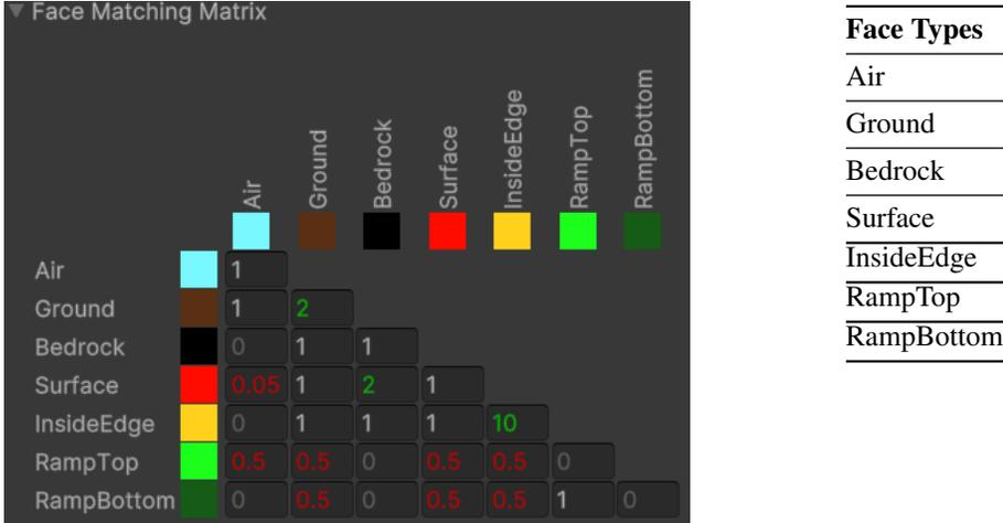
Figure 9: **Left:** The face matching matrix between face types in OpenXLand. **Right:** The face types in the adjacency matrix. Each metatile is made of tiles, which have faces, and the adjacency matrix determines which faces can be neighbors. The adjacency matrix constrains the set of permissible metatiles that can be placed at a given location during the environment generation process.
