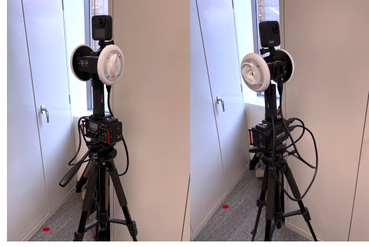
Figure 7: Recording system. It comprises a professional binaural microphone, a sports camera, and a recorder.
