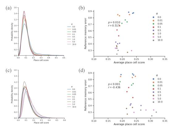
Figure S5: Place cell score analysis for non-recurrent positional embeddings for N = 32. Place cell score distributions with varying  $\alpha$  in self-attention layers (a) and feed-forward layers (c). Scatter plot of average place cell scores and reference memory errors for self-attention layers (b) and feed-forward layers (d). r and p denote Spearman's rank correlation coefficient and significance score, respectively.
