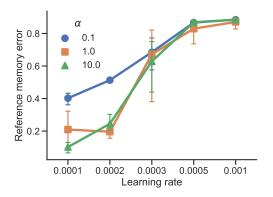
Figure S8: Familiar map reference memory error results with five different learning rates, where  $\alpha \in \{0.1, 1.0, 10.0\}$ , for a total of 64 training maps (N = 64). The error bars represent the standard deviation of errors from three independently trained models.
