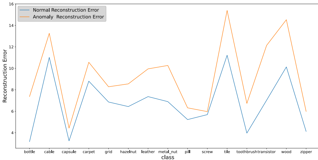
Figure 1: The average reconstruction error of normal and anomalous images of different categories in MVTec-AD.
