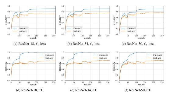
Figure 6: We apply ResNet-18, 34, 50 on noisy CIFAR-100 with both  $\ell_1$ -loss and cross-entropy loss (CE). The data generator and optimizer are the same as those in CIFAR-10 experiment. For each trial, we set the initial learning rate to be  $\eta = 0.05$  and run 260 epochs and decay the learning rate with factor 0.33 for each 50 epochs.
