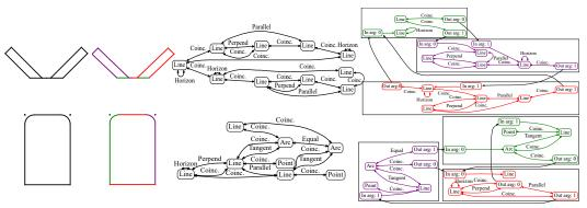
Figure 3: **Design intent parsing.** Left: input raw sketches and sketches restructured with concepts. Right: raw constraint graphs and modular constraint graphs. Primitives and constraints in the restructured sketches and graphs are colored according to concepts.
