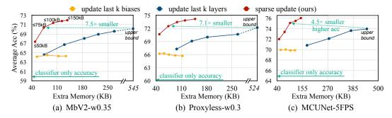
Figure 9. Sparse update can achieve higher transfer learning accuracy using 4.5- $7.5 \times$  smaller extra memory (analytic) compared to updating the last k layers. For classifier-only update, the accuracy is low due to limited capacity. Bias-only update can achieve a higher accuracy but plateaus soon.
