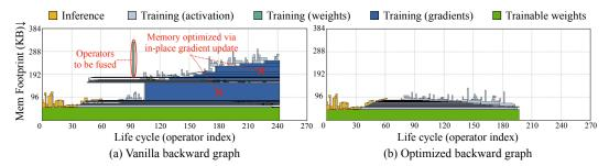
**Figure 7.** Memory footprint reduction by operator reordering. With operator reordering, TTE can apply in-place gradient update and perform operator fusion to avoid large intermediate tensors to reduce memory footprint. We profiled MobileNetV2-w0.35 in this figure (same as Figure 1).
