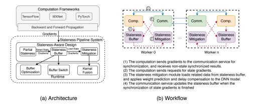
Figure 1: The architecture and workflow of SAPipe. Solid lines: data flow with all gradients. Dashed lines: data flow with stale gradients.
