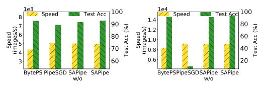
(a) VGG16 with partial staleness. "SAPipe w/o" de-(b) ResNet50 with partial staleness. "SAPipe w/o" notes SAPipe without partial staleness. denotes SAPipe without partial staleness.
