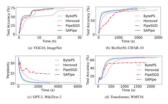
Figure 8: Convergence of different models. The x-axis is wall-clock training time, and the y-axis is perplexity (lower is better) for GPT-2, and test accuracy (higher is better) for others.
