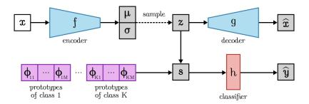
Figure 1: Schematic representation of the architecture of ProtoVAE. The input image x is encoded by f into a tuple  $(\mu, \sigma)$ . A vector z is sampled from  $\mathcal{N}(\mu, \sigma)$  which, on one side, is decoded by ginto the reconstructed input  $\hat{x}$  and, on the other side, is compared to the prototypes  $\phi_{kj}$  resulting in the similarity scores s. The latter are passed through the classifier h to get the final prediction  $\hat{y}$ .
