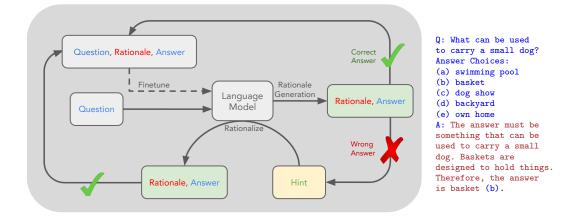
Figure 1: An overview of STaR and a STaR-generated rationale on CommonsenseQA. We indicate the fine-tuning outer loop with a dashed line. The questions and ground truth answers are expected to be present in the dataset, while the rationales are generated using STaR.
