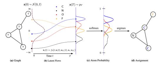
Figure 2: A demonstration of the modular flow generation. The initial Gaussian distributions  $\mathcal{N}(0, I)$  evolve into complex densities  $\mathbf{z}(T)$  under f and are subsequently translated into probabilities and labels.
