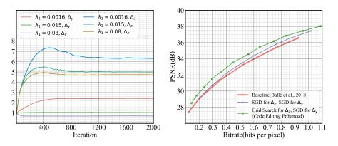
Figure A2: Comparison of gradient decent and grid search for optimizing  $\Delta_z$ . Left: the trend of  $\Delta_y$  and  $\Delta_z$  during gradient based optimization. Right: R-D performance comparison. SGD is the abbreviation of stochastic gradient descent, and in practical implementation we use Adam [Kingma and Ba, 2014] as optimizer.
