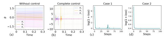
Figure 25: Dynamics of the state variables in the uncontrolled system (a) and in the controlled system using the complete control (b), initiating from  $(\theta_1, \theta_2, \theta_3, \dot{\theta}_1, \dot{\theta}_2, \dot{\theta}_3)|_{t=0} \sim \mathcal{N}(0, I_{6\times 6})$ . Logarithm of the training loss in case 1 using the complete control (c) and in case 2 using the partial control (d).
