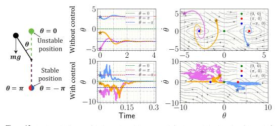
Figure 13: A schematic diagram of the inverted pendulum system (left), the sampled trajectories of the angle  $\theta$  (middle), and the corresponding orbits in the phase space (right).
