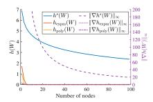
Figure 2: The values of  $h_{\rm expm}$  and  $h_{\rm poly}$  get very close to zero for a number of nodes as small as ten. In contrast, letting s=1.001, we observe that  $h_{\rm ldet}^s$  can stay away from zero even for a cycle graph of 100 nodes. Finally, we note a similar pattern for the entrywise  $\ell_{\infty}$  norm of the gradients.
