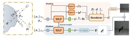
Figure 2: Overview of the method. For each camera ray, we first apply root-finding to locate the surface intersection point  $x_s$ .  $N_V$  points on the camera ray are sampled within a relatively large interval around the surface to generate accumulated shading values.  $N_L$  points are sampled on the surface-to-light segment to calculate the light visibility, which is multiplied to the accumulated shading to output the final RGB value.
