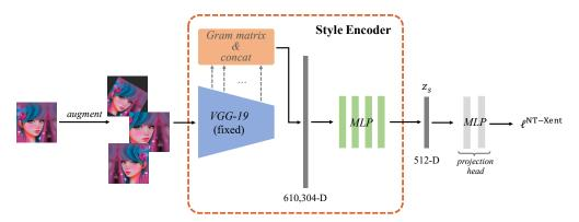
Figure 3: Architecture of the proposed style encoder, which consists of a pretrained *VGG-19* [46] network, a *Gram matrix and concat* module and an MLP predictor. More detailed notations are described in the contexts of Sec. 3.1.
