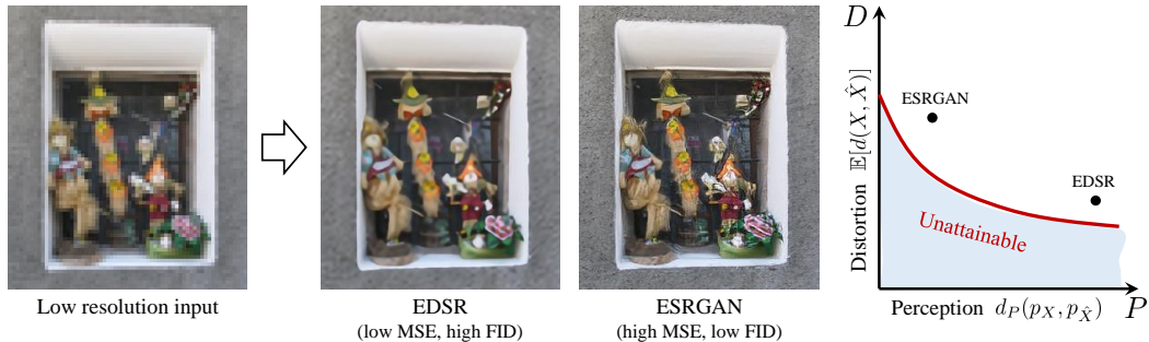
Figure 1: Illustration of the distortion-perception tradeoff in super-resolution. A low resolution image (left) is fed to two state-of-the-art super-resolution algorithms (middle). EDSR [14] achieves a low MSE distortion, but produces blurry reconstructions with high FID values [10]. ESRGAN [31] outputs photo-realistic recoveries with low FID, but its MSE is significantly higher. This is a result of the distortion-perception tradeoff (right). Namely, estimators cannot simultaneously achieve a low distortion and have their outputs distributed like the signals they are designed to estimate. In this paper, we derive a closed form expression for the distortion-perception function (red curve) for the MSE distortion and Wasserstein-2 perception index.
