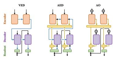
Figure 1: Schematic of the three primary architectures analyzed in this work. The orange, purple, and green boxes represent the encoder RNNs, decoder RNNs, and linear readout layers, respectively. Recurrent connections are shown in blue, attention-based connections and computational blocks are shown in gold. The grey circles add positional encoding to the inputs.
