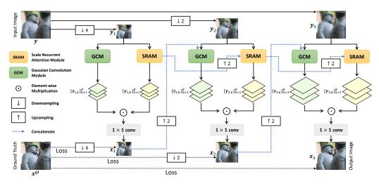
Figure 1: Diagram of proposed GKMNet for SIDD with T = 3.
