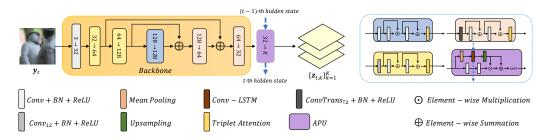
Figure 2: Diagram of SRAM. All convolutional kernels are of size  $3 \times 3$ .
