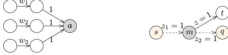
Figure 4: (left) There are three weights encoding w_1 , w_2 , and w_3 . They are all connected to the output vertex a . (right) For each middle neuron m , we add an input neuron s and the edges sm and m q with weights z_1 and z_2 .
