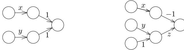
Figure 2: (left) The architecture of the subtraction gadget. The data point d = (1, 1; 0) enforces that the constraint x = -y .
