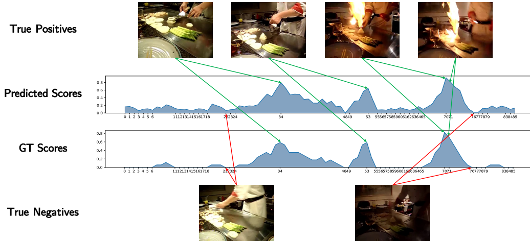
Figure 4: Qualitative result comparing the generic summary from CLIP-It with the ground-truth summary. The plots showing predicted and ground-truth frame-level scores are similar, indicating that frames that were given a high score in ground-truth were also assigned high scores by our model.
