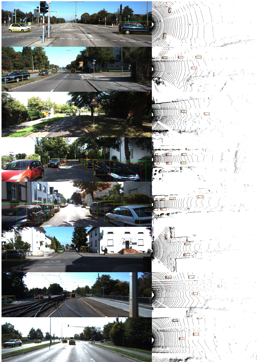
Figure 2: More qualitative results on the KITTI validation dataset. The 3D ground-truth boxes and our predictions are drawn in green and red, respectively. We demonstrate the results in various scenarios with different lighting conditions and occlusions, including cities, residential districts and roads.
