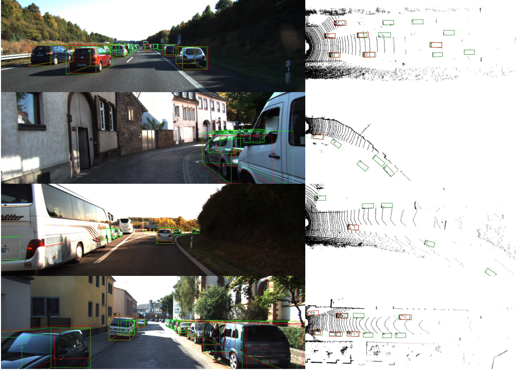
(a) Bad case in our methods. Low recall rate of the 2D detector is shown.
