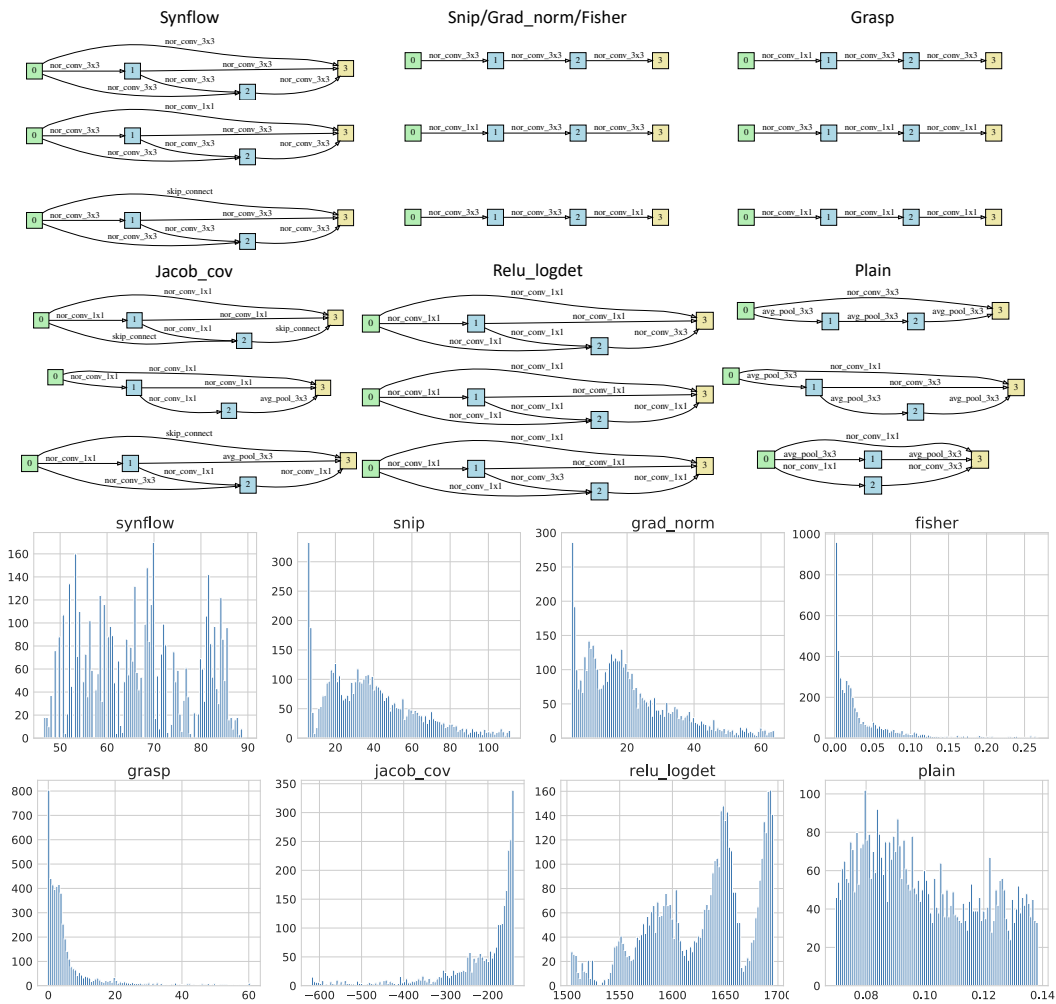
Figure A25: Top: Top-3 zero-shot ranked architectures on NB201. Bottom: Histogram of zero-shot scores. For synflow , we plot the histogram of the log values of synflow scores (varying from 0 to 7.55 \times 10^{49} ). Since there are many outliers in all types of zero-shot scores, only the histogram of the zero-shot scores between the 0.1 and 0.9 quantile are plotted.
