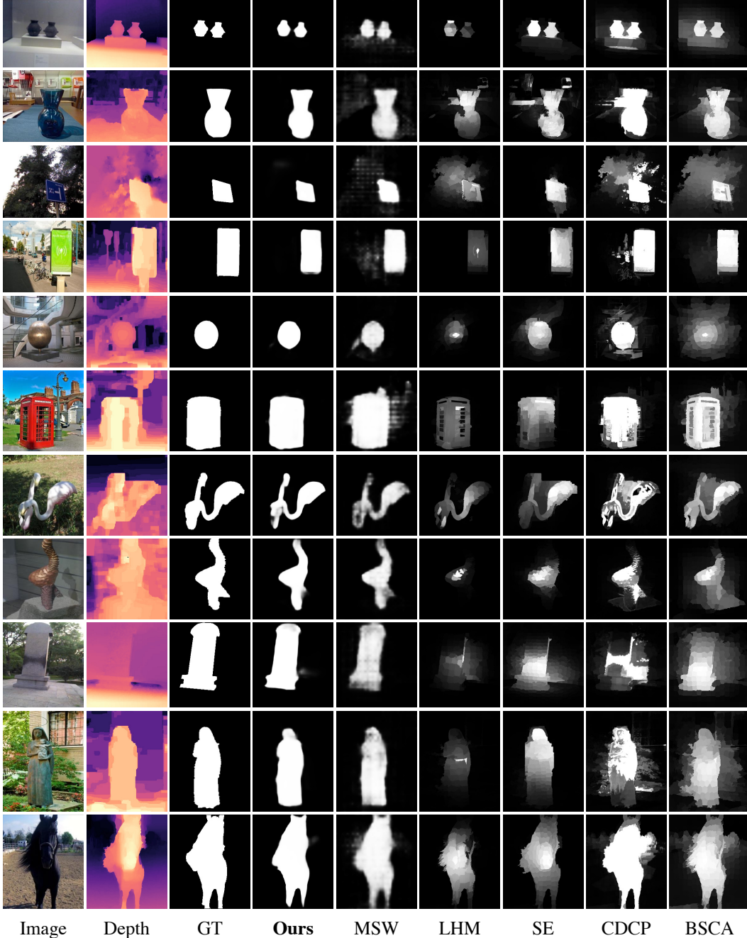
Figure 3: Visual comparisons of weakly-supervised and unsupervised saliency models. ‘GT’ represents the ground-truth saliency for reference only.
