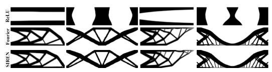
Figure 10: We use different network architectures to parameterize both the density and displacement field. Since the ReLU-MLP fails to capture the high-frequency details, its solution for the forward problem is far from being accurate, resulting in meaningless structures for the inverse problems. Fourier feature and SIREN networks produced similar results, thus, suitable for our method.
