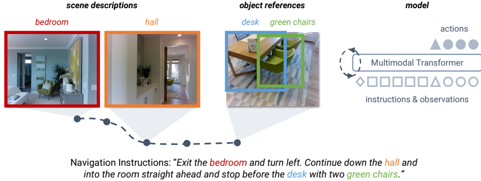
Figure 1: Illustrative VLN Instruction. Visual landmarks in the instruction include scene descriptions (e.g., ‘bedroom’ and ‘hall’) and object references (e.g., ‘desk’ and ‘green chairs’). Unlike most previous methods, our model uses both scene ( \Delta ) and object features ( \odot ) to match the visual references in the instructions. We employ a novel attention mechanism and view aggregation strategy to select the most relevant features for action prediction.
