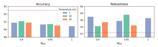
(b) Effect of  $\alpha_{kld}$  and temperature  $\gamma$  on accuracy and robustness. The dotted red line represents training without soft labels (i.e.,  $\alpha_{kld} = 0$ ).
