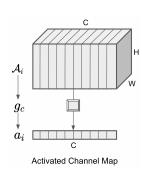
Figure 5: Mapping function  $g_c$  is applied channelwise to get the Activated Channel Maps (ACM).
