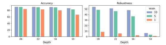
(a) The figure shows effect of decreasing number of layers and number of channels on accuracy and robustness for our method. The teacher model is a robust WideResNet-28-10 and student models are WideResNet-Depth-Width.
