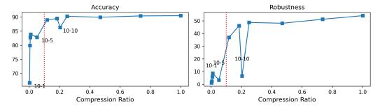
(b) The figure shows compression ration vs accuracy and robustness for our method. The dotted red line represents compression ratio of 0.1. Our method works in transferring robustness beyond this point except for dips caused by WideResNet of depth 10.
