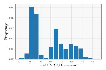
Figure S7: Number of msMINRES iterations needed to achieve a relative residual of  $10^{-3}$ . Histogram captures training a M = 5,000 SVGP model on the 3droad dataset (subsampled to 30,000 data points).
