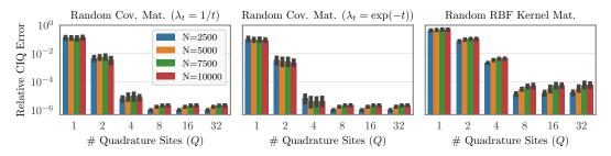
Figure S1: CIQ relative error at computing  $\mathbf{K}^{1/2}\mathbf{b}$  as a function of number of quadrature points Q. In all cases Q = 8 achieves  $< 10^{-4}$  error.
