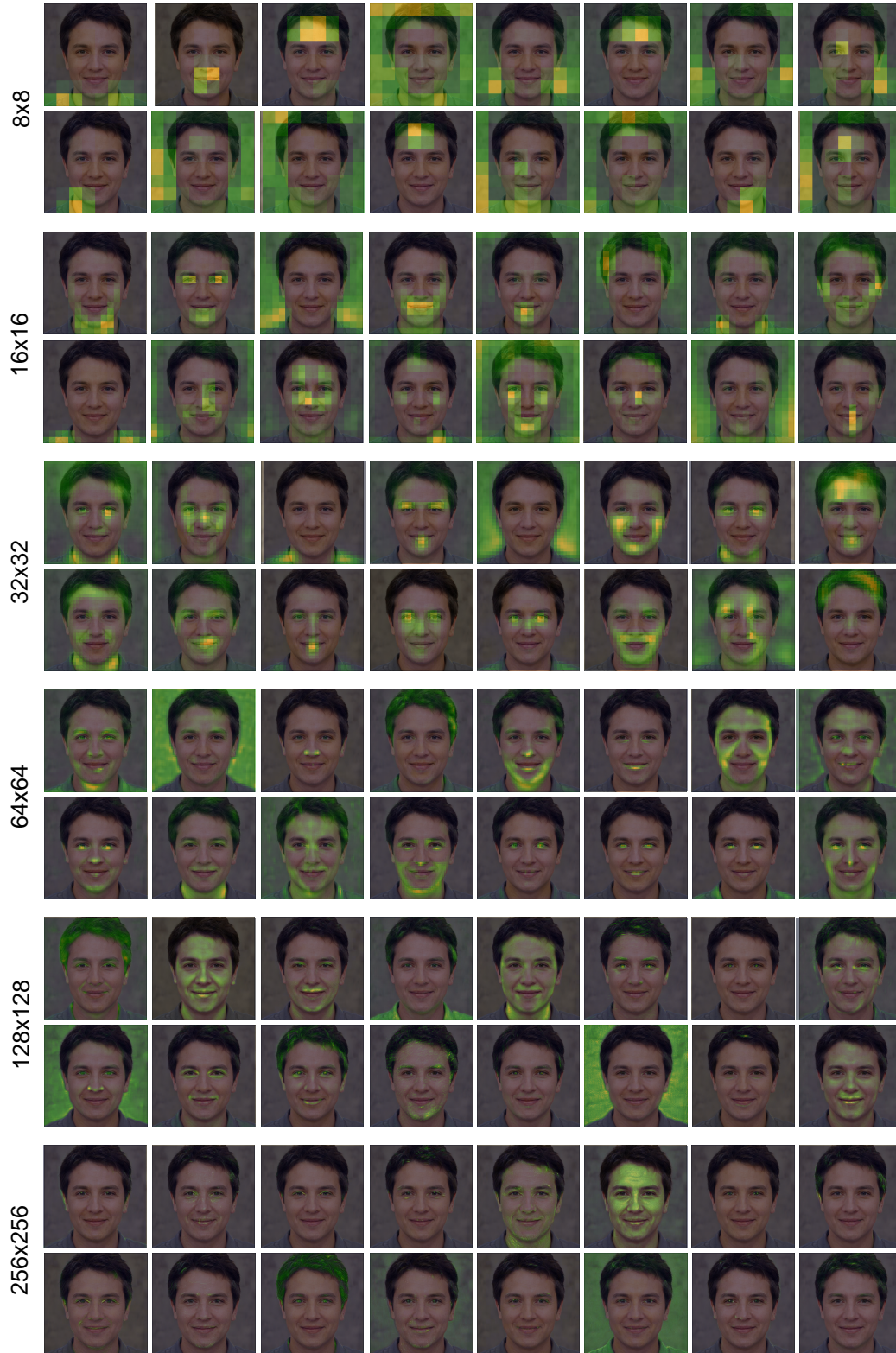
Figure 1: Visualization of the semantics learned in different resolutions. We show 16 groups in each layer with the resolution increasing from 8 \times 8 to 256 \times 256 . The attention maps are obtained by averaging the feature maps in a group. It can be observed that features with low resolutions (i.e., 8 \times 8 - 64 \times 64 ) show better performance in learning semantics (e.g., eyes, mouths and hair).
