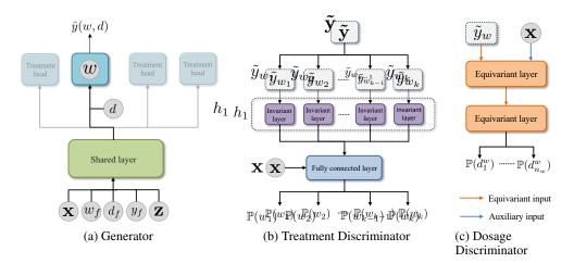
Figure 3: Architecture of our generator and discriminators.
