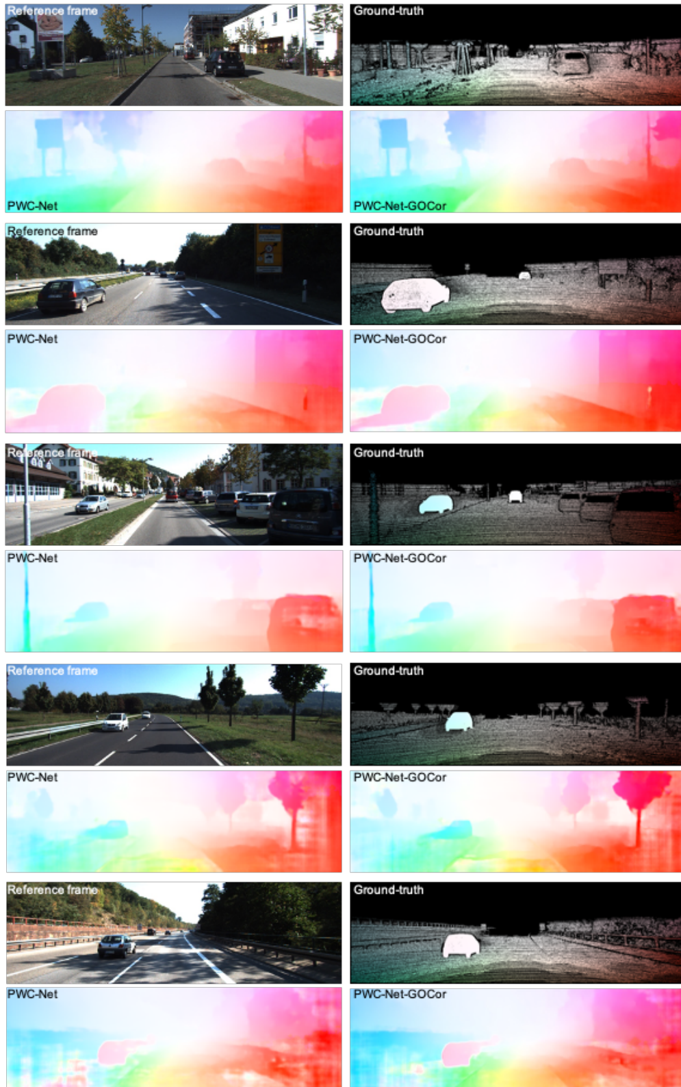
Figure 8: Qualitative examples of PWC-Net and PWC-Net-GOCor applied to images of KITTI-2012 and KITTI-2015. Both models are trained on Flying-Chairs followed by 3D-Things .
