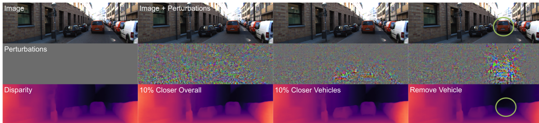
Figure 1: Altering the predicted scene with adversarial perturbations. Top to bottom: input image; adversarial perturbations with upper norm of 2 \times 10^{-2} ; predicted scene visualized as disparity. Left to right: original image and predicted scene; overall scene altered to be 10% closer; all vehicles altered to be 10% closer; vehicle in the center of the road is removed by perturbations.
