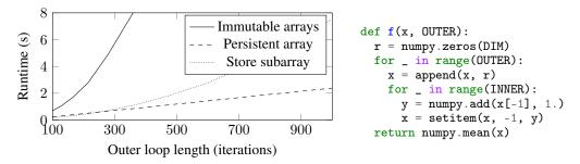
Listing 8: Runtime for a simplified version of a lattice language model with dimension 2000 and inner loop of 15 iterations. Results are an average of 10 runs.
