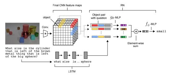
Figure 2: **Visual QA architecture**. Questions are processed with an LSTM to produce a question embedding, and images are processed with a CNN to produce a set of objects for the RN. Objects (three examples illustrated here in yellow, red, and blue) are constructed using feature-map vectors from the convolved image. The RN considers relations across all pairs of objects, conditioned on the question embedding, and integrates all these relations to answer the question.
