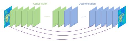
**Figure 1:** The overall architecture of our proposed network. The network contains layers of symmetric convolution (encoder) and deconvolution (decoder). Skip-layer connections are connected every a few (in our experiments, two) layers.
