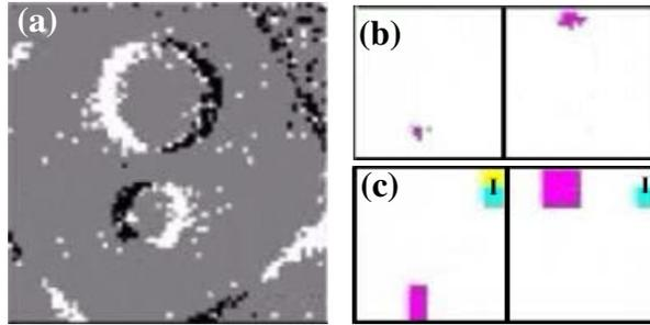
**Fig. 8: Captured AER outputs at different stages of processing chain. (a) at the retina output, (b) at the output of the 2 convolution chips, (c) at the output of the object chip. 'I' labels the activity of the inhibitory neurons.**
