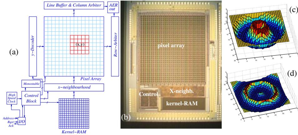
**Fig. 3. Convolution chip (a) architecture of the convolution chip. (b) microphotograph of fabricated chip. (c) kernel for detecting circumferences of radius close to 4 pixels and (d) close to 9 pixels.**
