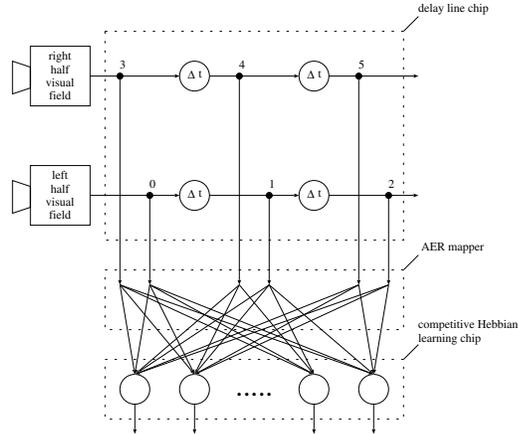
**Fig. 5: System setup for learning direction of motion**
