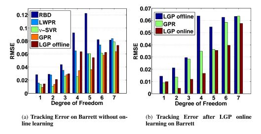
Figure 5: (a) Tracking error as RMSE on test trajectory for each DoF with Barrett WAM. (b) Tracking error after online learning with LGP. The model uncertainty is reduced with online learning using LGP. With online learning, LGP is able to outperform offline learned models using standard GPR for test trajectories.
