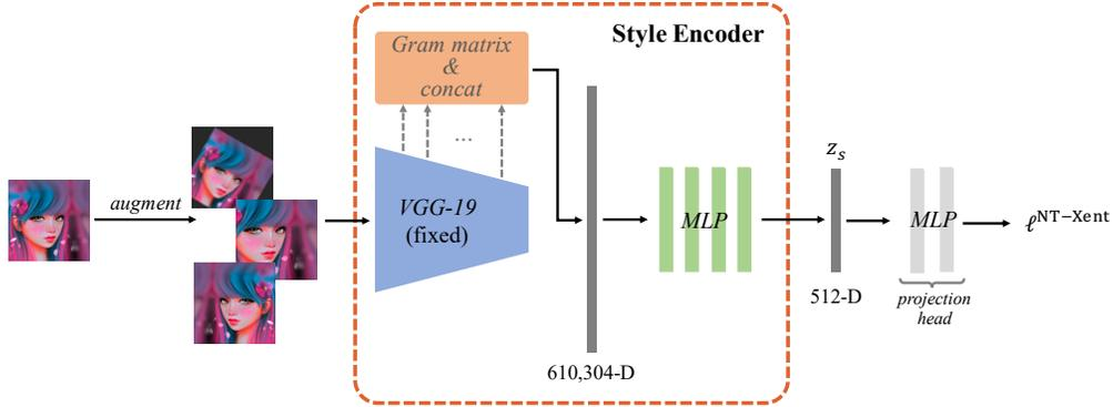
Figure 3: Architecture of the proposed style encoder, which consists of a pretrained VGG-19 [46] network, a *Gram matrix and concat* module and an MLP predictor. More detailed notations are described in the contexts of Sec. 3.1.
