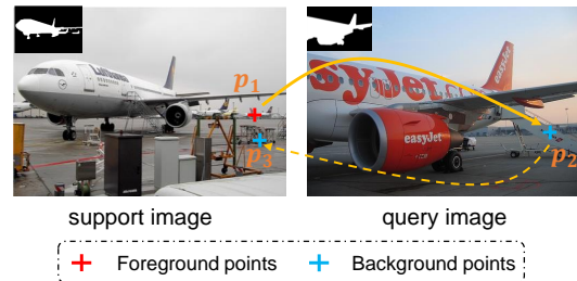
Figure 2: The motivation of our proposed method. Many pixel-level support features are quite different from the query ones, and thus may confuse the attention. We incorporate cycle-consistency into attention to filter such confusing support features. Note that the confusing support features may come from foreground and background.
