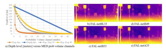
Figure 2: Effects of exponential disparity discretization.
