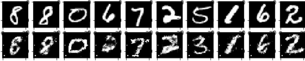
Figure 1: VEEGAN method can be used like ALI to perform inference. The means output from the reconstructor network for the real images in the top row are used as the latent features to samples the generated images in the bottom row.
