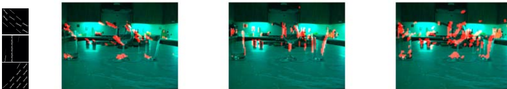
Figure 3: Detected quantized transparent local features (transparent visual words) on an example image. Each image shows the detected locations for the transparent visual word corresponding to the latent topics depicted on the left.
