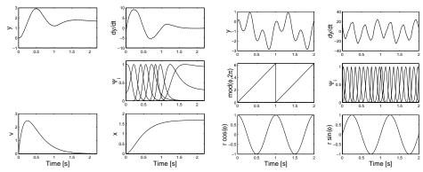
Figure 1: Examples of time evolution of the discrete CPs (left) and rhythmic CPs (right). The parameters  $\mathbf{w}_i$  have been adjusted to fit  $\dot{y}_{demo}(t) = 10\sin(2\pi t)\exp(-t^2)$  for the discrete CPs and  $\dot{y}_{demo}(t) = 2\pi\cos(2\pi t) - 6\pi\sin(6\pi t)$  for the rhythmic CPs.
