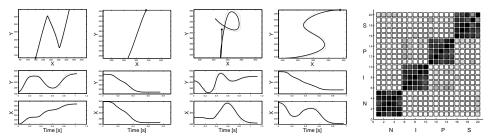
Figure 4: Left: Examples of two-dimensional trajectories fitted by the CPs. The demonstrated and fitted trajectories are shown with dotted and continuous lines, respectively. **Right:** Correlation between the weight vectors of the 20 characters (5 of each letter) fitted by the system. The gray scale is proportional to the correlation, with black corresponding to a correlation of +1 (max. correlation) and white to a correlation of 0 or smaller.
