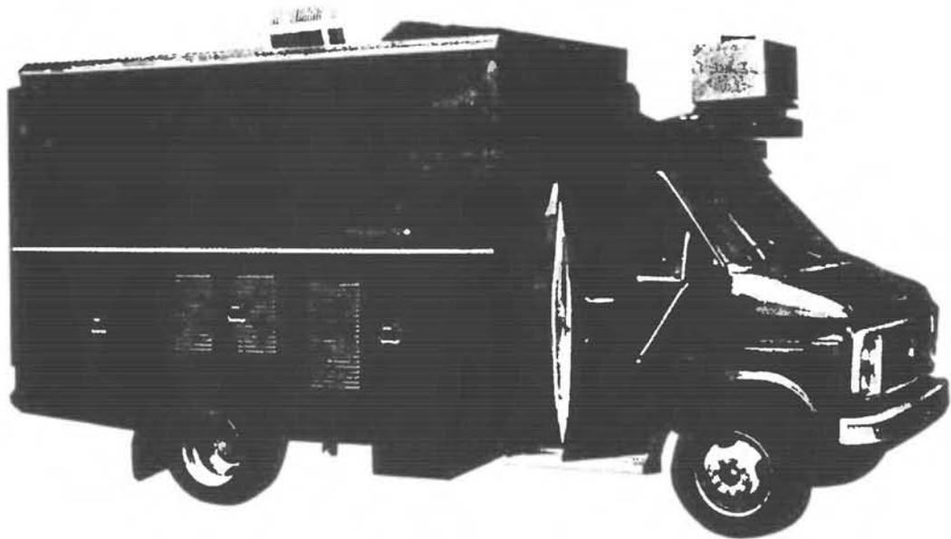
Figure 3: NAVLAB, the CMU autonomous navigation test vehicle.
